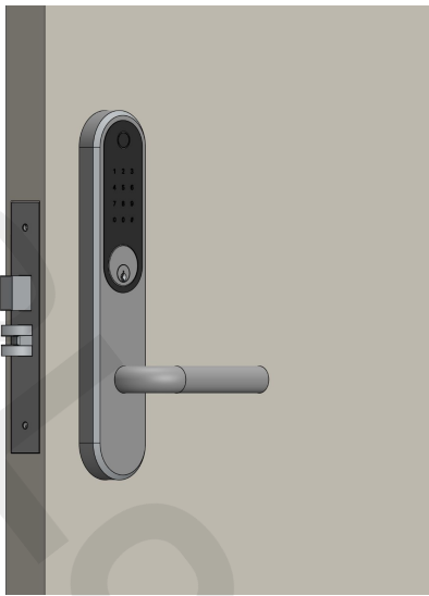
13) Slide the faceplate over the bolt and latch and secure with the small 6mm screws
